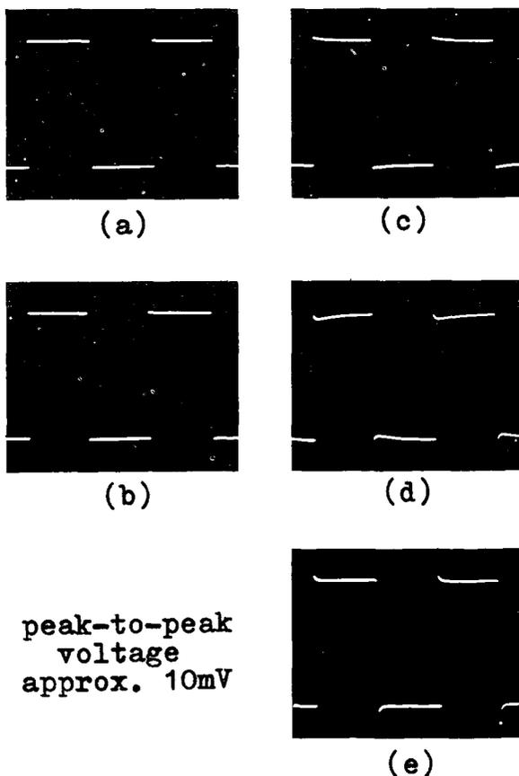
Fig. 6. Output waveforms from circuit of Fig. 3, fed from Levell TG200DM square-wave source via circuit of Fig. 5. (a) 1000 Hz, all values as calculated. (b) 50 Hz, all values as calculated. (c) 1000 Hz,  $R_4$  5% low. (d) 50 Hz,  $C_1$  5% high. (e) 50 Hz,  $R_2$  5% high.
