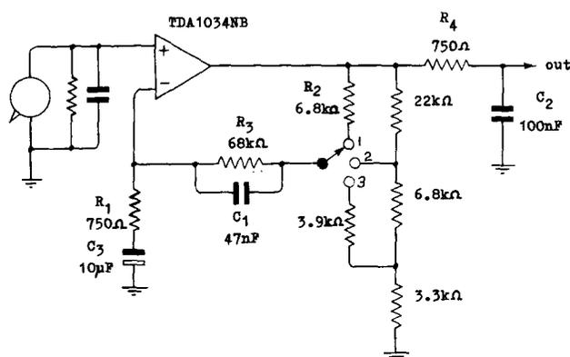
Fig. 3. Practical design for disk input circuit.
