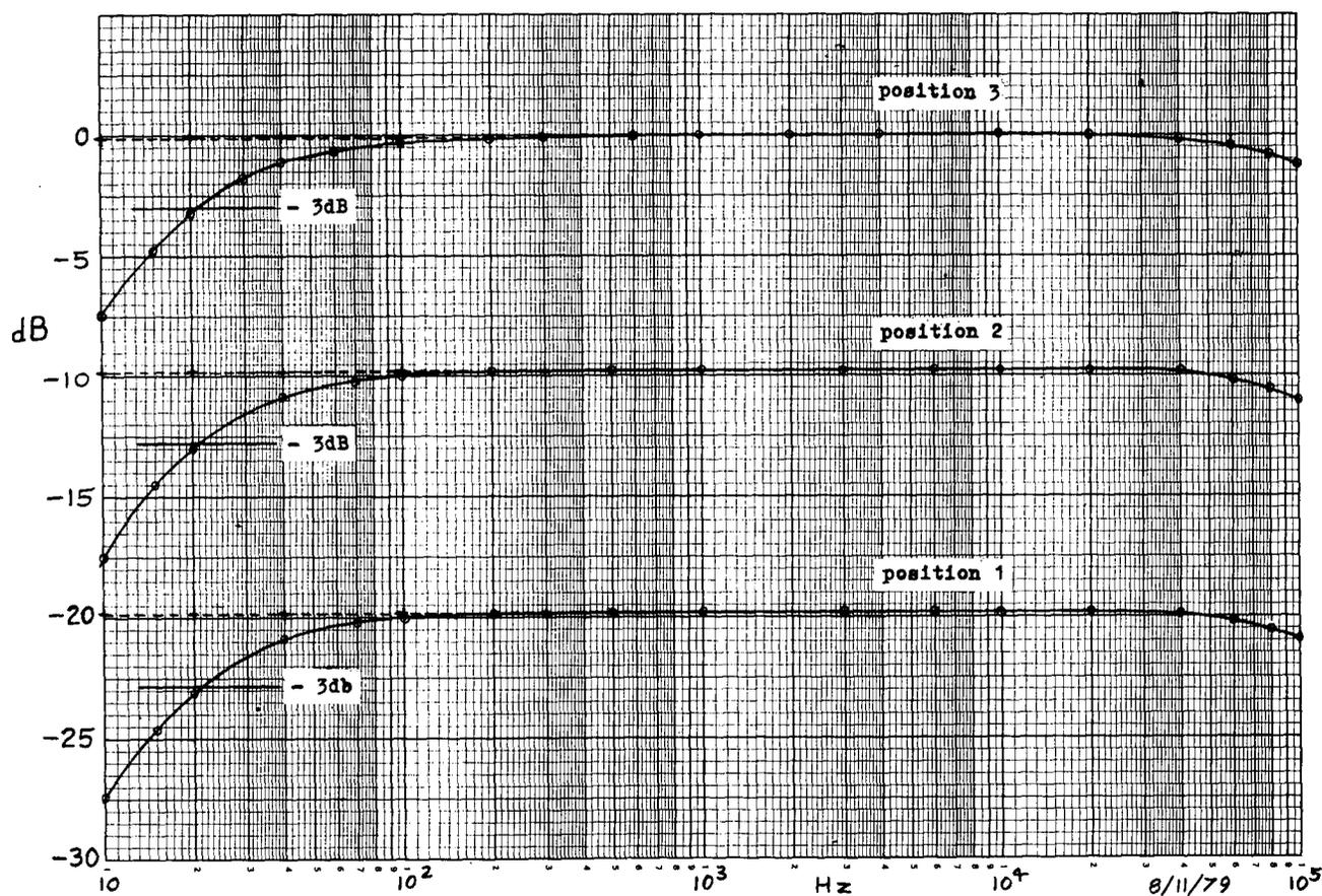
Fig. 4. Measured response curves for Fig. 3 circuit. The broken-line curves were obtained with  $C_3$  short-circuited.
