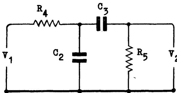
Fig. 7. Circuit for providing 7950- $\mu$ s and 75- $\mu$ s time constants.
